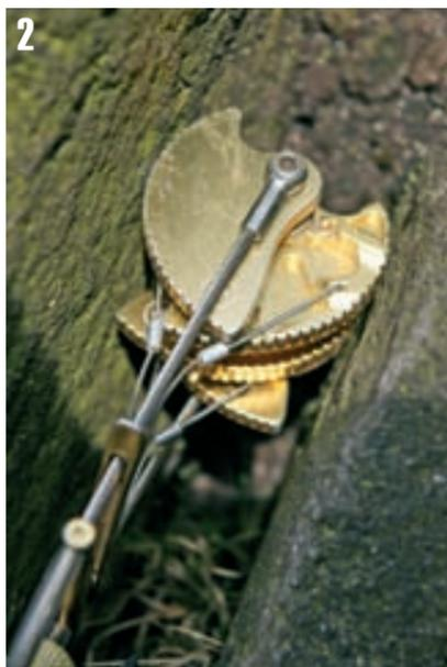
in a crack may feel reassuring but this isn't allowing it to work effectively and in addition often results in it getting jammed solid. *Photo 2* shows a badly over-cammed placement.
